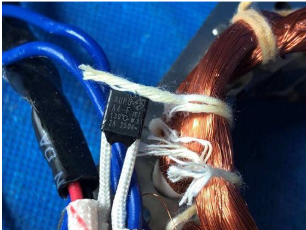
Thermal link built in fan motor
