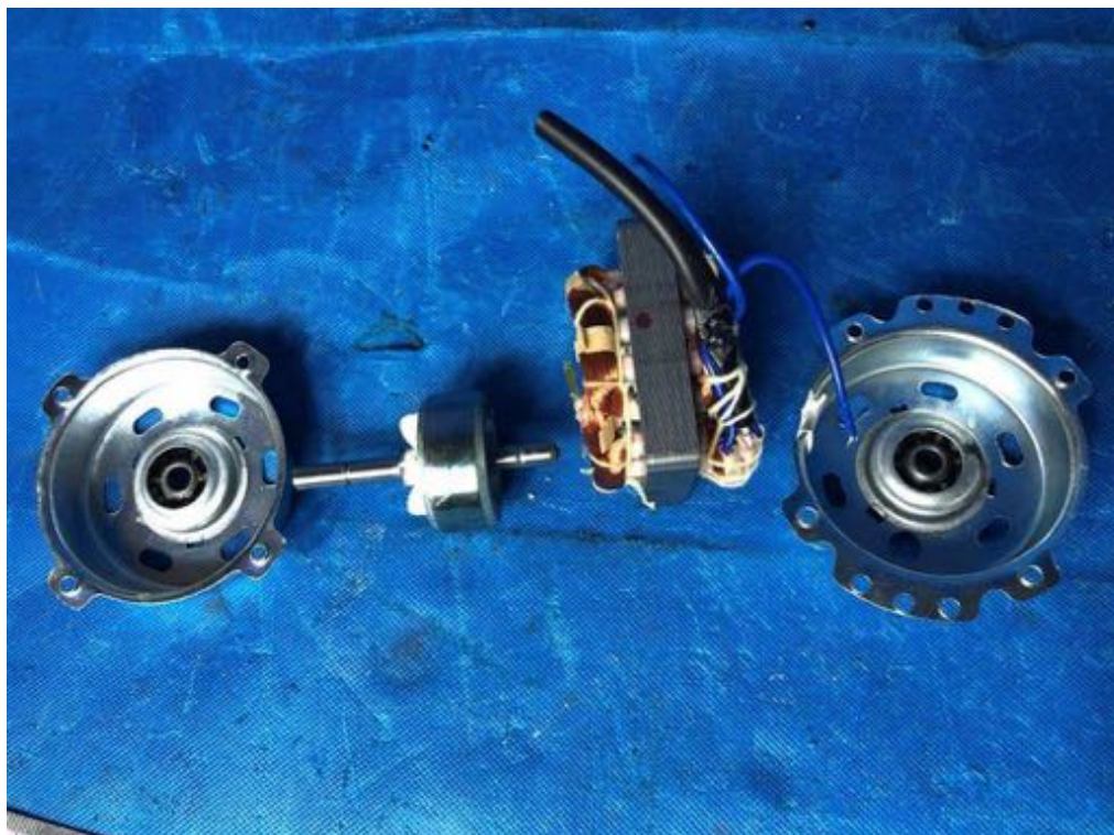
Internal view of fan motor
